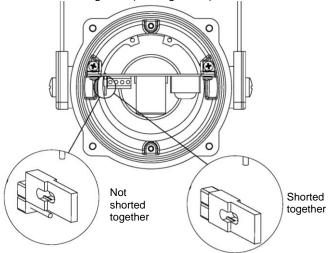
Fig. 10 Header Pin Settings
