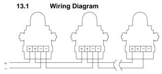
Fig. 7 DC Simplified Block Diagram (negative switching)
