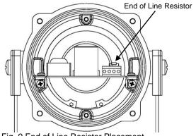
Fig. 9 End of Line Resistor Placement
