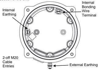
Fig. 3 Internal View of Cover
