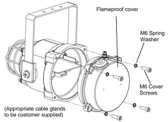
Fig. 2 Accessing the Explosion proof Enclosure.
