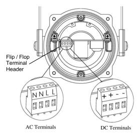
Fig. 4 Internal View of BExBGD 5 Joule Beacon
