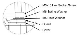
Fig. 13 Cover and Guard Fixtures
