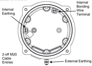
Fig. 3 Internal View of Cover
