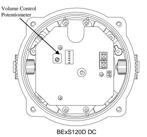
Fig. 9 Location of Volume Control Potentiometer
