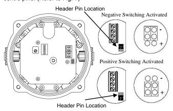
Fig. 7 Stage Switching Polarity
