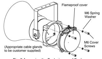
Fig. 2 Accessing the Explosion proof Enclosure.
