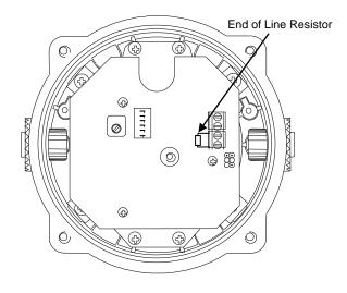
Fig. 7 End of Line Resistor Placement
