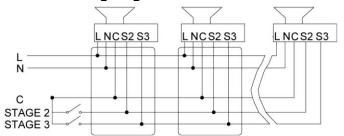
Fig 3. BExS120 AC Simplified Block Diagram
